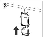
**Step 6.** Install a Bus Cable End Cap at the end of AC bus cable
